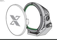
**LENS PROTECTOR REMOVAL** Remove lens protector by unclipping the side wings.
